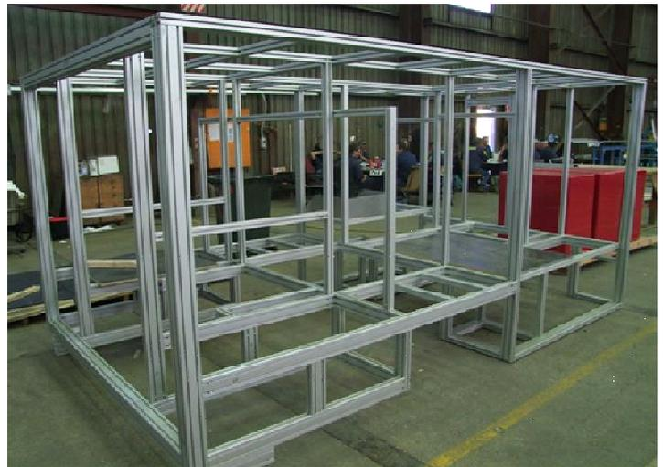
There are 350 individual connection points on this frame with a saving of between 300% to 500% in labour costs using Alusic standard connectors.
