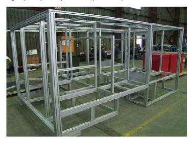
There are 350 individual connection points on this frame with a saving of between 300% to 500% in labour costs using Alusic standard connectors.
